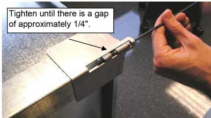
Figure 27: Tighten Cap Screw to 1/4" of the Coupling
